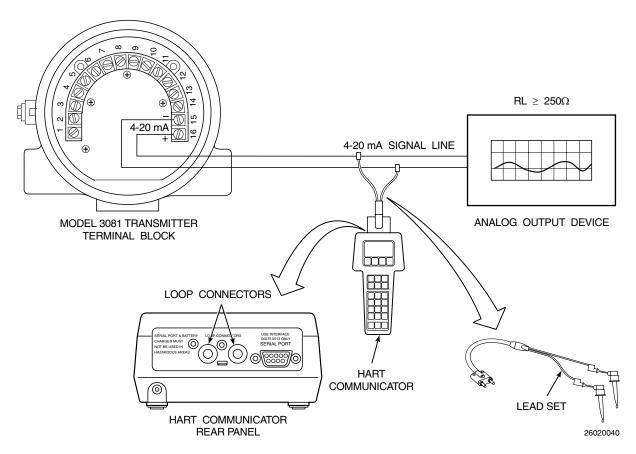
Figure 4-1. Signal Line Connections, ≥ 250 Ohms Lead Resistance
